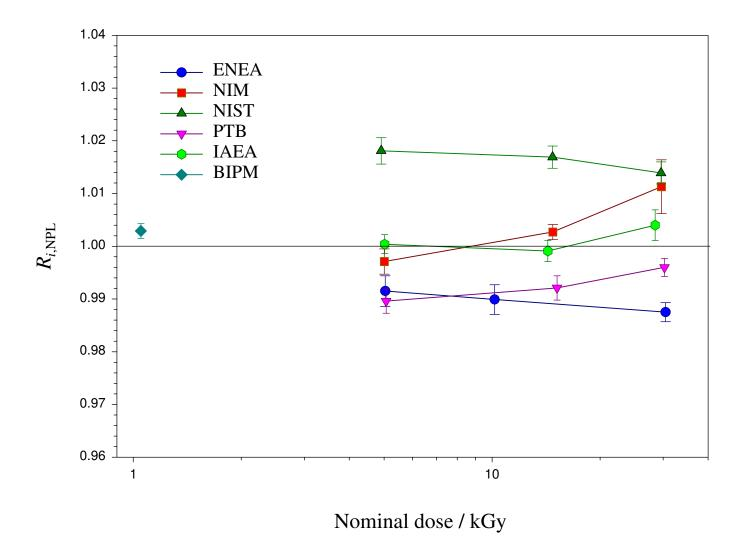
Figure 2. Results for the comparison ratios  $R_{i,\mathrm{NPL}}$  using the alanine transfer dosimeter of the NPL. The uncertainty bars represent the statistical standard uncertainty  $s_{i,\mathrm{NPL}}$ .
